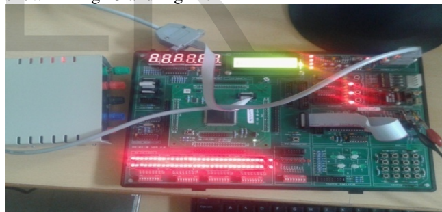
Figure 23. FPGA Implementation of QPSK modulation proposed method -2
