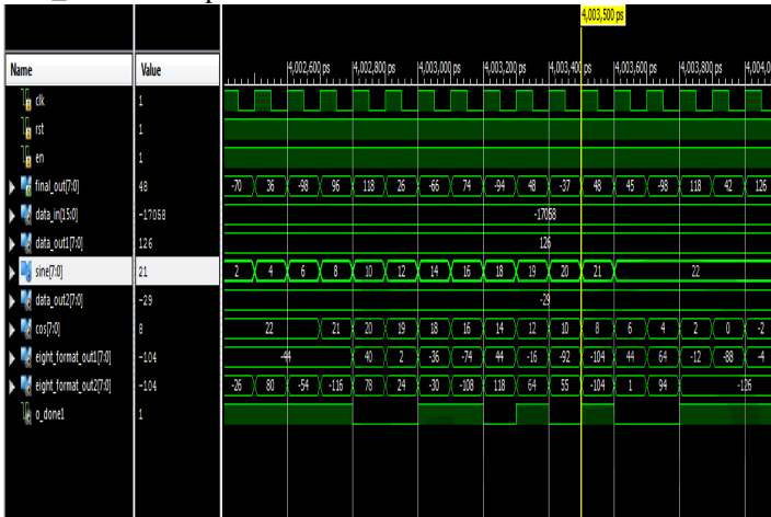
Figure 15. QPSK modulation for proposed method-1 in ISim simulator with AWGN.
